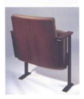
**SEAT:** The seat inner panel shall be ply-wood. The padding shall be glued to the inner panel, and shall conform to the CA TB 117. The seat shall have a built-in counter-weight to insure automatic self-rising without the aid of springs. The seat shall be fully upholstered on all surfaces and enclosed at the rear/bottom with a zipper allowing on-site re-upholstery.
